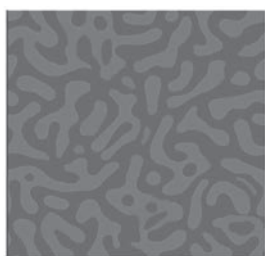
Figure 4 A representation of the typical random phase separation structure of polymer blend systems.
