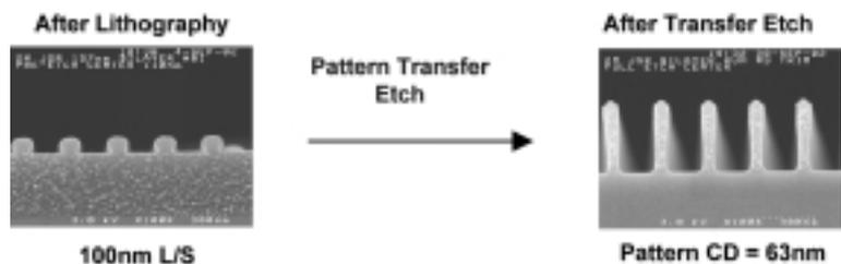
Fig. 4 JSR ArF Spin-on SHM Process: 63nm Patterning Result
