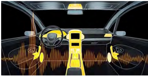
Points where squeaks are effectively suppressed by using HUSHLOY™
