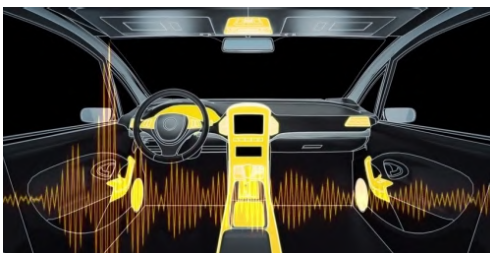
Points where squeaks are effectively suppressed by using HUSHLLOY™
