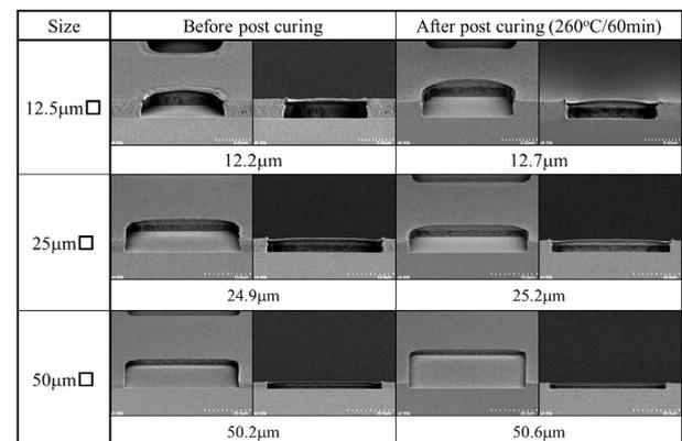
Figure 3 SEM images of the patterns before and after post curing.
