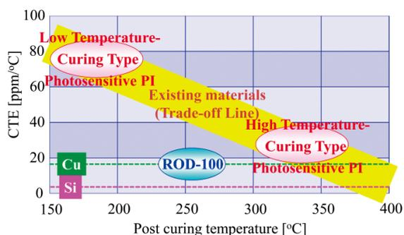
Figure 1 Correlations of CTE and curing temperature.
