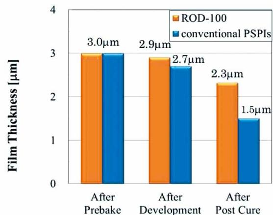
Figure 4 Film thickness change through process.
