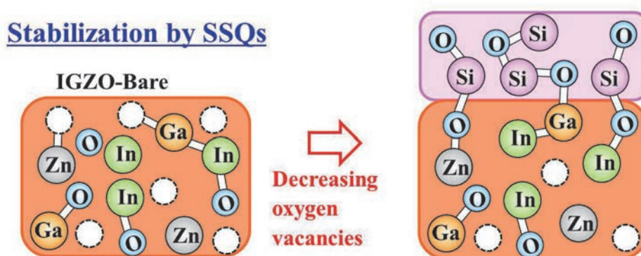
Figure 9 Schematic images for stabilization mechanism of IGZO by SSQs.
