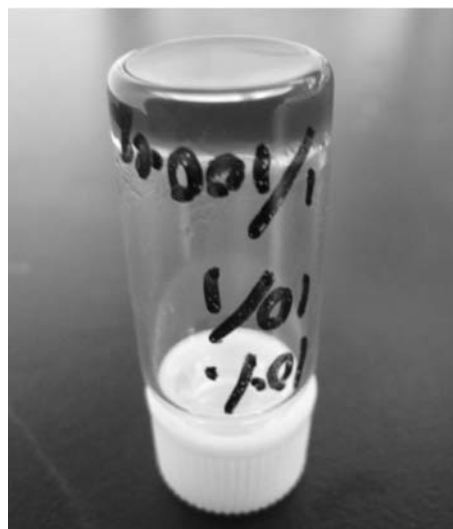
Figure 4 Photograph of the GPE obtained by Pt-catalyzed polymerization of SBMC/HMBS in a electrolyte solution ( [\text{SBMC}]/[\text{HMBS}]=10/1 , total monomer concentration:10wt%, electrolyte solution:1 M LiPF 6 -EC/DEC(3/7))
