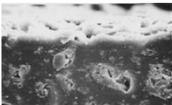
Fig. 7 SEM image of cut sample of JSR standard pad after soaking in water for 24hrs.
