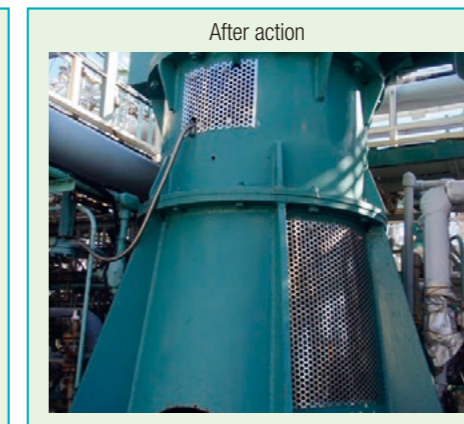
A protective cover (perforated metal) was installed to prevent people from getting caught in the agitator shaft
